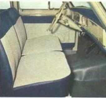
The rear seat and its back rest fold down to provide more space for loading goods according to requirements. The loading floor is dismountable so that it case of need a large space is available to bulkier goods.
